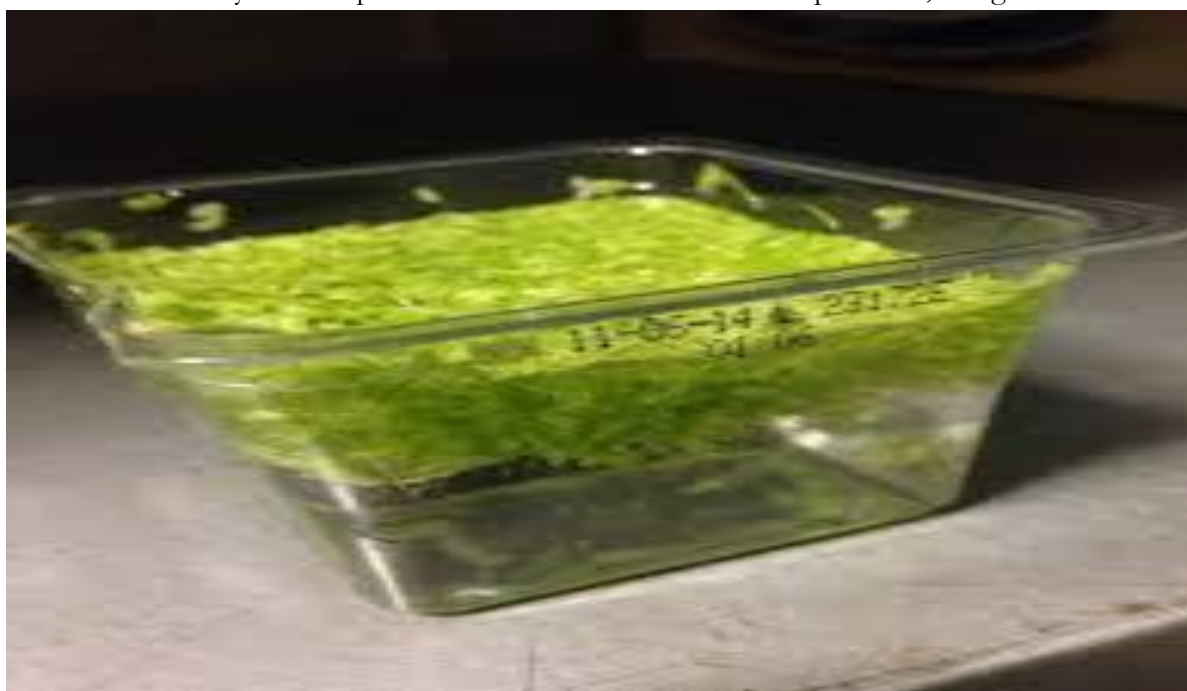
Figure 1: Use of the aquatic plant Lemna minor L. for the reduction of pollutants in pulp and paper mill effluent in laboratory
